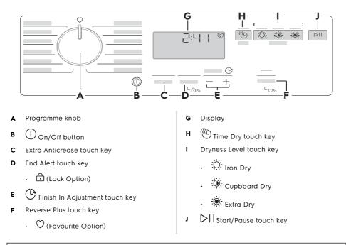
(1) Press the touch buttons with your finger in the area with the symbol or name of the option. Do not wear gloves when you operate the control panel. Make sure that the control panel is always clean and dry.
