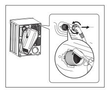
Re-install the inlet hose. Make sure that the couplings are tight to prevent leakages.
